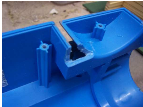
Footplate re-built with packers, refitted buffer beam & part-footplate, some relieving needed for clearances.
