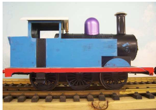
Rear bunker was cut down lower, buffer beam raised, Cab cut-outs, bigger roof plate, chimney & done enlarged.
