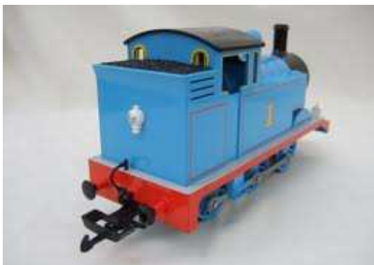
Rear bunker was cut down lower, buffer beam raised, Cab cut-outs, bigger roof plate, chimney & done enlarged.
